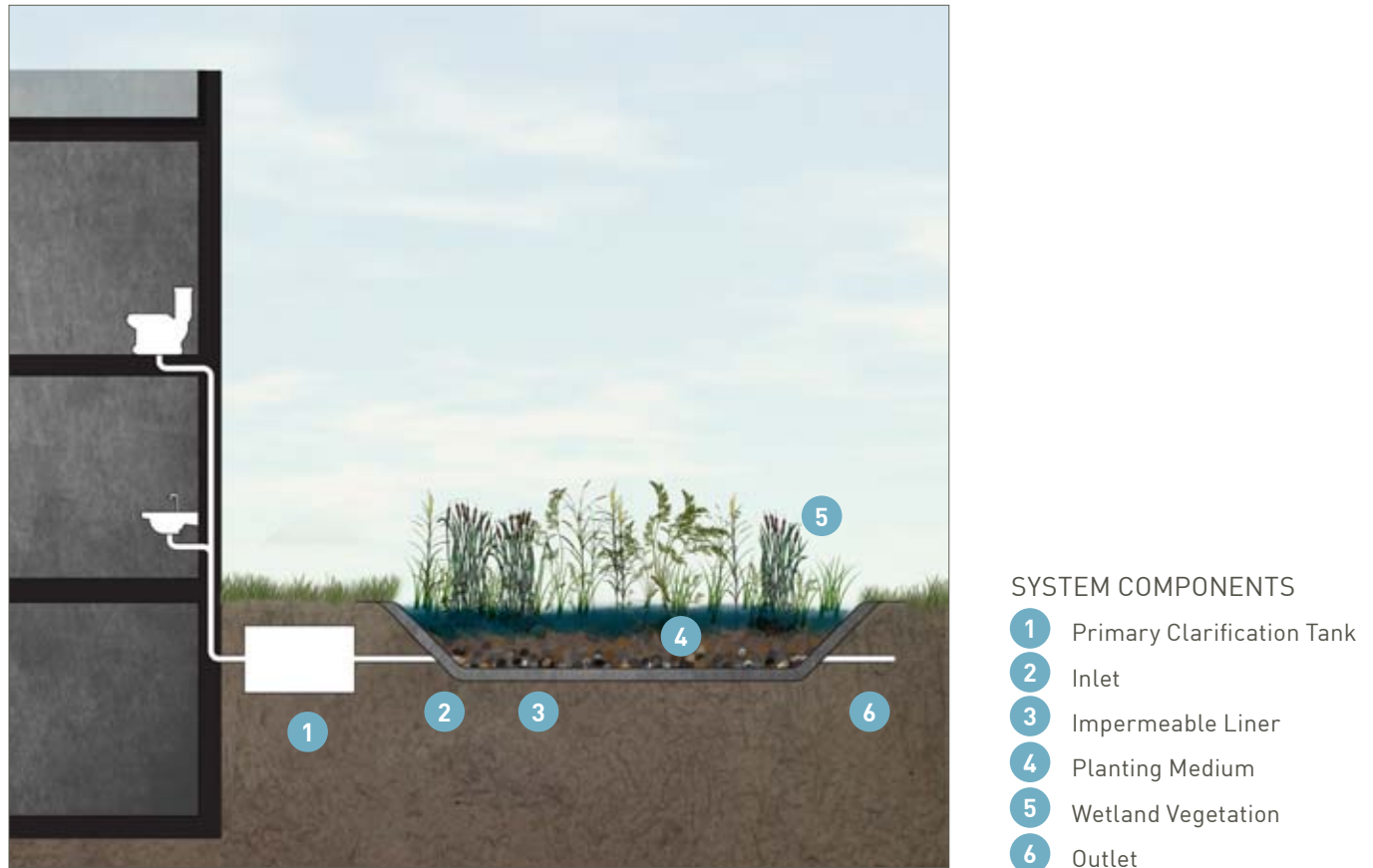
FIGURE W-2: CONSTRUCTED WETLAND
